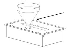
To filling the burner you have to push down the fuel cover.
