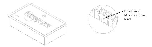
We advise to all users to fill the burner only to the bars mark (like you can see in the picture) Its capacity is define to support 2 litres.
