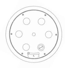
2 – Min. Position In that position it provides 6 hours of heat with only 2 litres of bioethanol;
