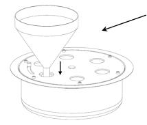
To filling the burner you have to push down the feeder. Then you have a small opening to put bioethanol. When you finish the process let it go and the feeder closed.
