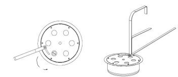
To regulate the flame of your burner you must with the help of the key move to the desired position.
