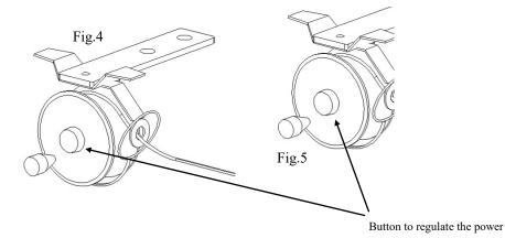
Unroll the two rear hub and then fix in the both sides of the pool in the axis chosen (Roll/Unroll the Button power.)
