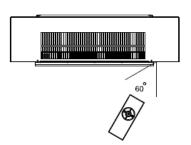
On the control panel, Switch A (see Fig.2) must be in the 'ON' (I) position in order for the remote control to operate. There are 3 buttons on the remote control. (See Fig.7) To operate correctly the remote handset must be pointed towards the heater outlet. (See Fig 12). The remote control functions are as follows:
